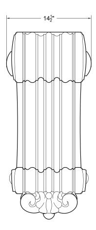
In order to facilitate release of castings from molds it is necessary to apply draft to certain edges/sides of castings. Casting tolerance is +/- 1/8 inch. For questions regarding draft or tolerance contact your product consultant. CDI retains ownership of all molds and patterns. Due to space constraints, molds can not be stored indefinitely. Please inform your product consultant if you plan to use this product for future projects. ©2017 Concrete Designs Inc. All rights reserved.
